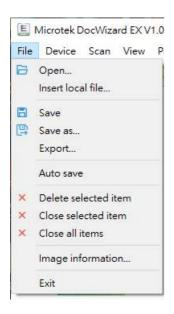
**A. Open:** Loads one or multiple files into the application; the opened file(s) will be added to the end of the list automatically.
