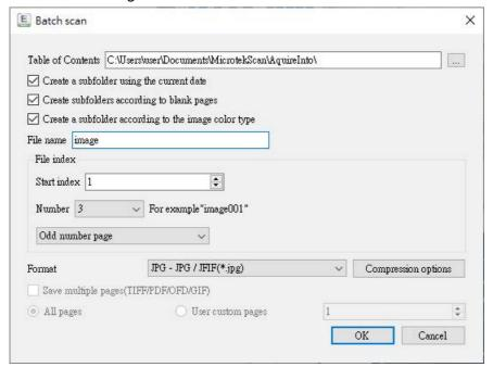
Click the "OK" button after finished setting the parameters and the scanner will perform batch scan. The scanned images will be saved into the specified folder automatically.
